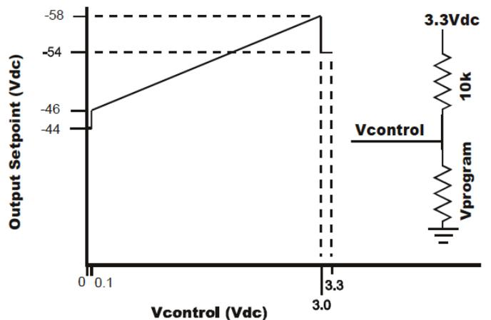
An open circuit on this pin reverts the voltage level back to the factory default setting.
